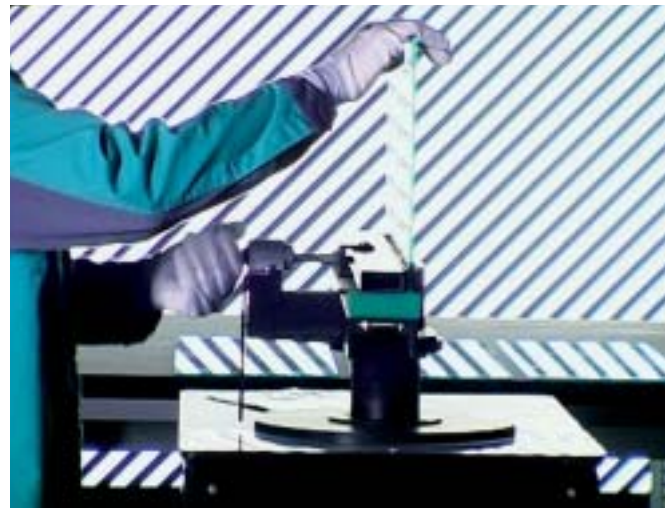
In the "zebra test", planarity (distortion) is checked at random.
