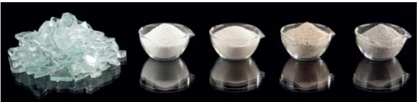
Raw materials used in float glass production (recycled fragments, soda, quartz sand, lime, dolomite)
